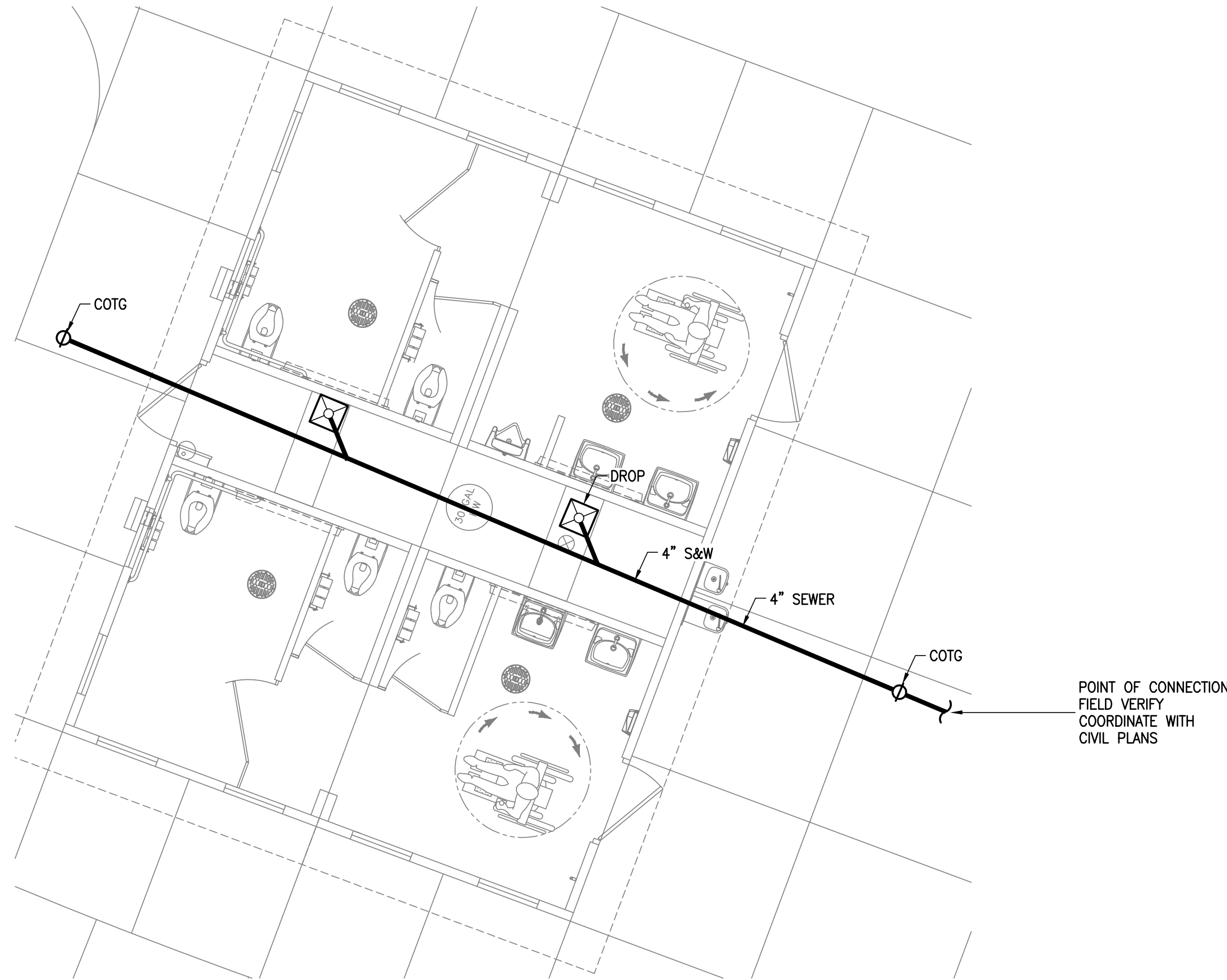
③ PLUMBING FLOOR PLAN RESTROOM BUILDING BELOW GROUND SCALE: 1/4" = 1'-0"
