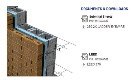
The most common modular brick heights are 2-1/4", 3-5/8", and 7-5/8". The brick that everyone is familiar with is 2-1/4" plus 3/8" mortar joint and three bricks and three mortar joints equals 8". Actually it adds up to 7-7/8", but either the mason makes up the 1/8" difference or the bricks are actually slightly larger. In either event you don't have to worry about it - it always works out to 8". The typical lengths are 8", 12" and 16". The usual width is 3-5/8".
