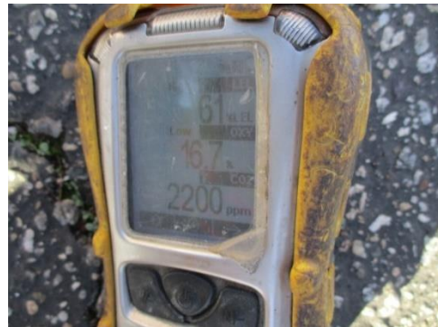
PID was used to test ambient air for worker safety and to measure soil gasses for prior to soil vapor testing.
