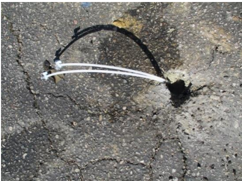
Nested vapor probes from boring B1.
