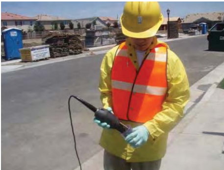
Figure D-6 Inserting meter into sample container
