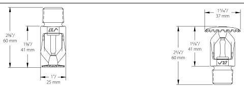
Standard Pendent with/without standard V9 coupling – V2707, V2708 Standard Upright with/without standard V9 coupling – V2703, V2704
