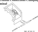
An uninsulated section of a single conductor should not be looped around the terminal and serve as two separate connections. The wire must be severed, thereby providing supervision of the connection in the event that the wire become dislodged from under the terminal. Failure to sever the wire may render the device inoperable risking severe property damage and loss of life.
